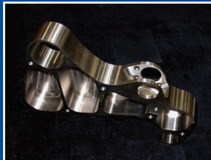
Machined Aerospace Part Material: Titanium
