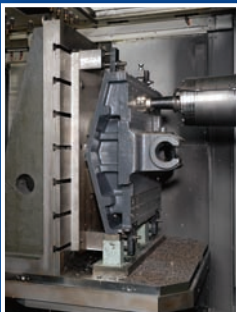
Machining Table Material: Gray Cast Iron
