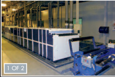
Chemcut SG540-40, 40" Continuous Etch-Strip Lines
