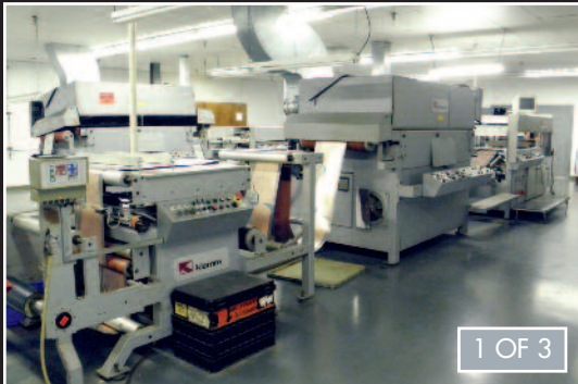
Numerous Klemm Continuous Reel to Reel Flex Circuit Screen Print Lines
